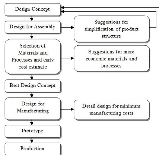
Fig. 3. The steps applying DfMA methods [6]
