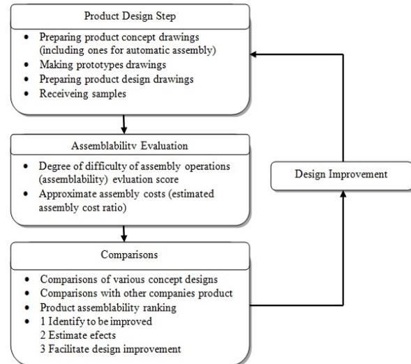
Fig. 5. Assessment of suitability for assembly and redesign [7]
