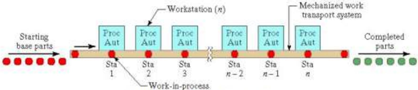
Figure 1 In-line configuration
